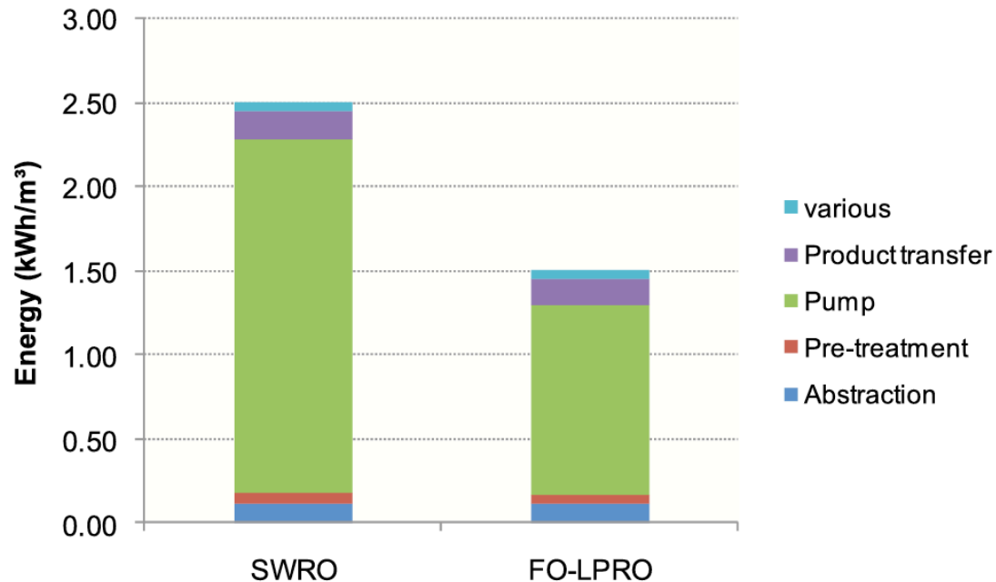
Figure 2.3.8 Comparison of energy consumption between desalination with RO and desalination with immersed FO-LPRO.
